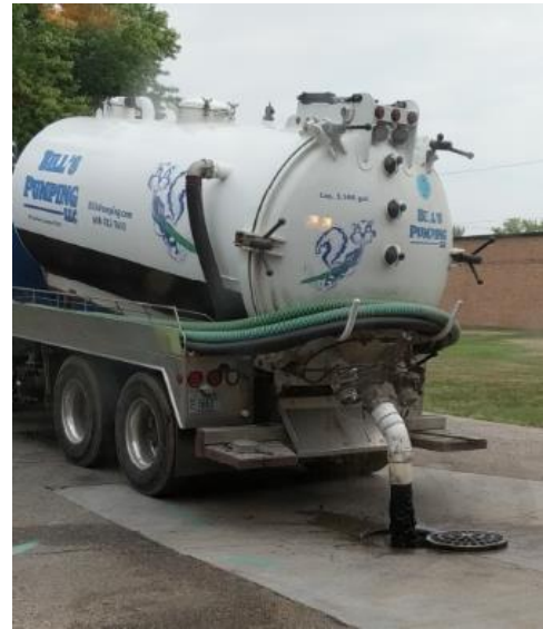
Figure 11 - Existing Septage Receiving
